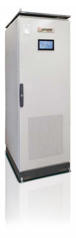
TITANIUM PLUS 2R-SCR rectifier series belongs to the Double Branch category thus provided with two independent AC/DC converters, one powering the direct current loads with stabilized voltage and the other dedicated to the battery charging.
