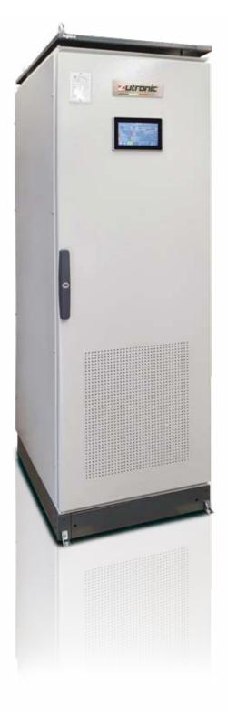
TITANIUM PLUS 2RP-SCR rectifier series belongs to the Double Branch category thus provided with two independent AC/DC converters in redundant (or power), parallel configuration, that supply the current loads and simultaneously charges a battery. They can be combined with vented/ sealed (VRLA) Lead Acid and Ni/Cd batteries.
