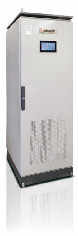
TITANIUM PLUS 2RP-CH rectifier series belongs to the Double Branch category thus provided with two independent AC/DC converters in redundant (or power), parallel configuration, that supply the current loads and simultaneously charges a battery. They can be combined with vented/sealed (VRLA) Lead Acid and Ni/Cd batteries.
